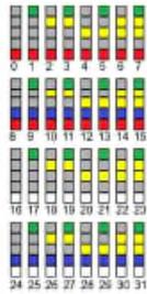
flow chart for setting the charging characteristic without graphic display
