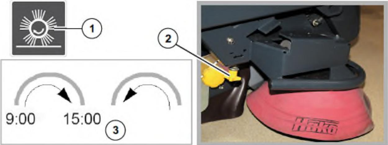
Check broom aprons (sealing strips) for clearance, wear and damage
