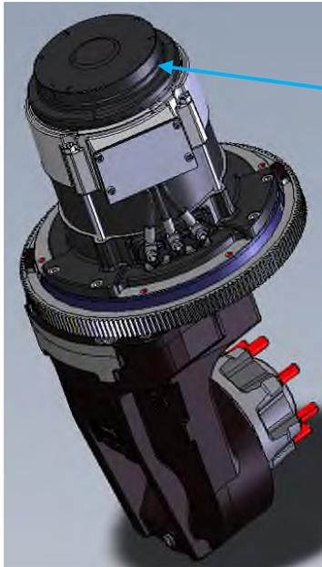
Front wheel drive parking brake can only be unlocked electrically (with tool kit 01381500)
