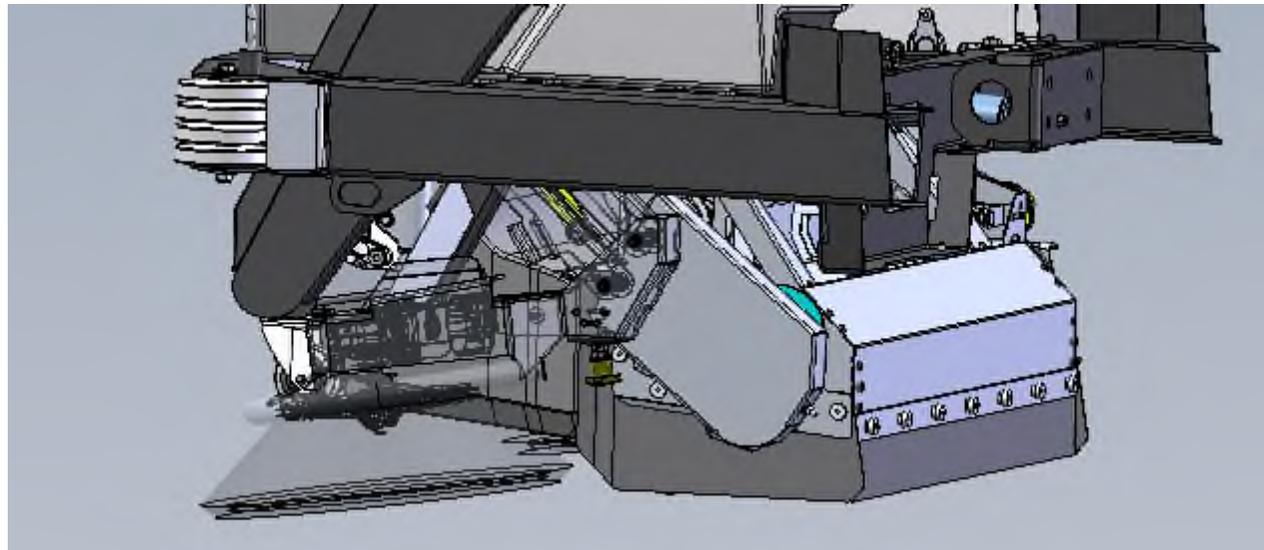
side and rear sealing strips 3 +/-1mm distance to the ground, this creates a negative pressure of approx. 0.5 mbar in the broom tunnel
