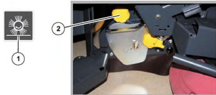
Check side broom for wear and damage
