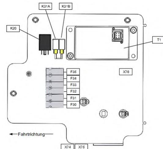
Checking of all power connections on the controls, drive control, power relays, fuses, potential distributors
